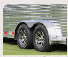
Aluminum construction of Sooner Select trailers features stout, durable triple hollow core sidewalls. The trailer is built with 2" x 4" 1-beams on 13" centers, meeting the demands of transporting livestock across the country.
