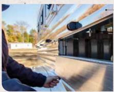
Lower air gaps with hinged cover panels on models with drop down windows allow for more air movement directly on the livestock.
